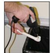
Figure 1.2-1: Drilling Elbow Hole over a Wastebasket
